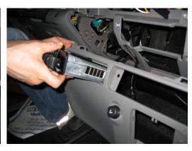
Remove brake control switch from lower trim panel. This will reinstall into console. (Equipment bracket sold separately)
